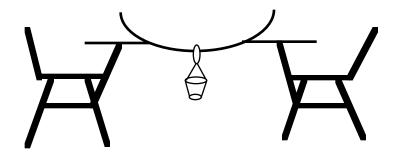
**Collecting Data:** Find the breaking weight for pieces of pasta that span gaps of different lengths – from 2 - 6 inches. Then try thicker "bridges" by using 2, 3, 4, and 5 strands of pasta. Record the (length, strands, weight) data in a table like this.
